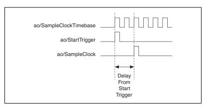
Figure 5-6. ao/SampleClock and ao/StartTrigger
